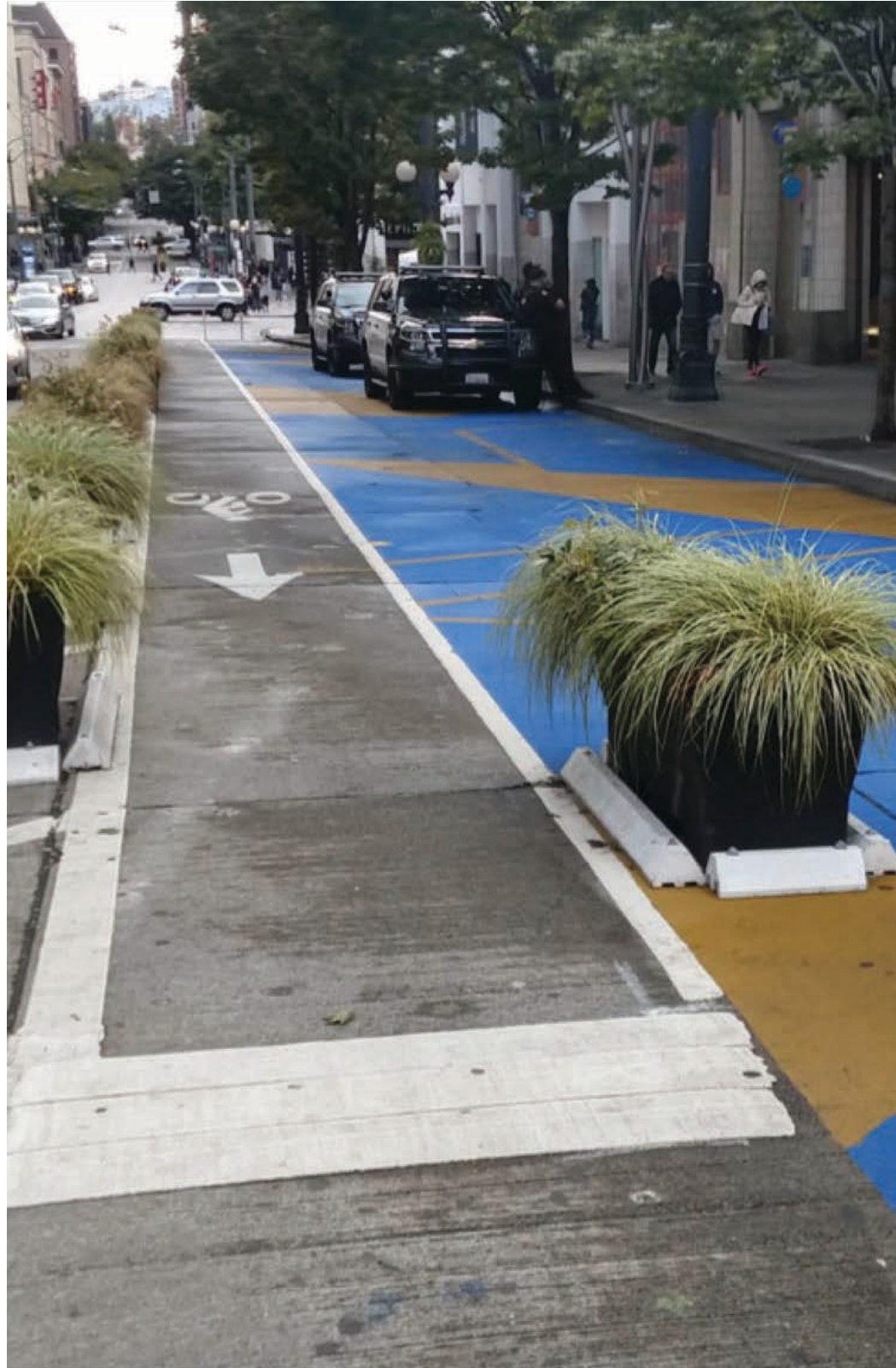
Figure 6. Protected bike lanes provide clear guidance for bikes and for service or ride share vehicles, ensuring safe movement for all.
